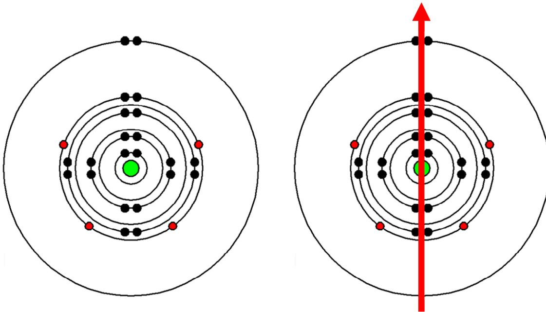
When several billion iron atoms are in a group where their tiny magnets are all lined up in the same direction, this is called a magnetic domain. A bar of iron will be made up of billions and billions of magnetic domains.
