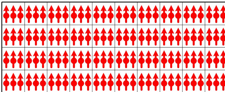
Some materials, when exposed to a strong external magnetic field, will allow their domains to line up and stay lined up even after the field is removed. This would be called a hard magnetic material, and permanent magnets are made from this. Examples are Alnico (aluminum, nickel, cobalt and iron), NdFeB (neodymium, iron,
