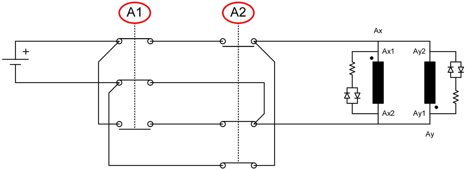
Showing how the switches were wired, since each coil was fed with its own pair of wires.
