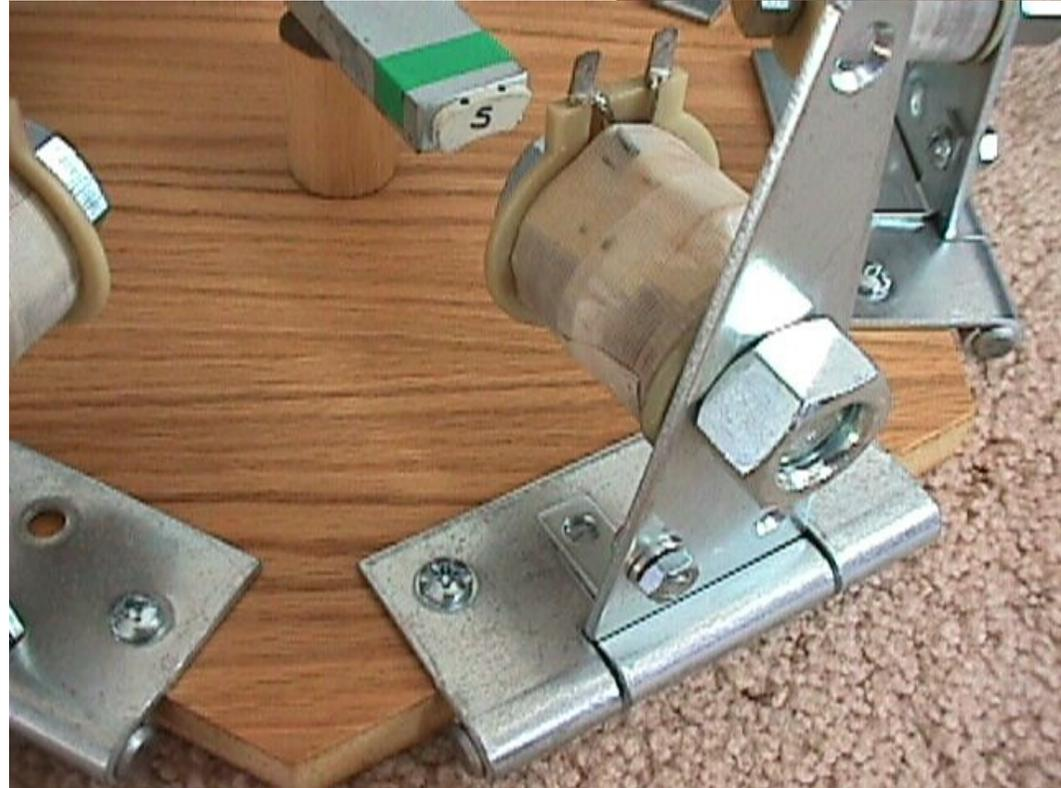
I used brass strip and small L bracket to hold hinges upright
